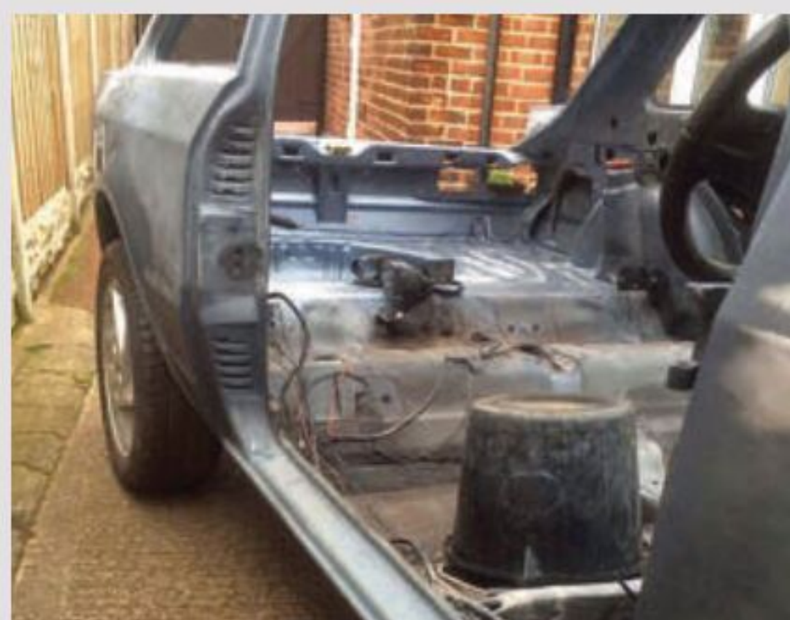
Once stripped, Andrew found the bodyshell was pretty good, but it still needed complete sills on both sides.
