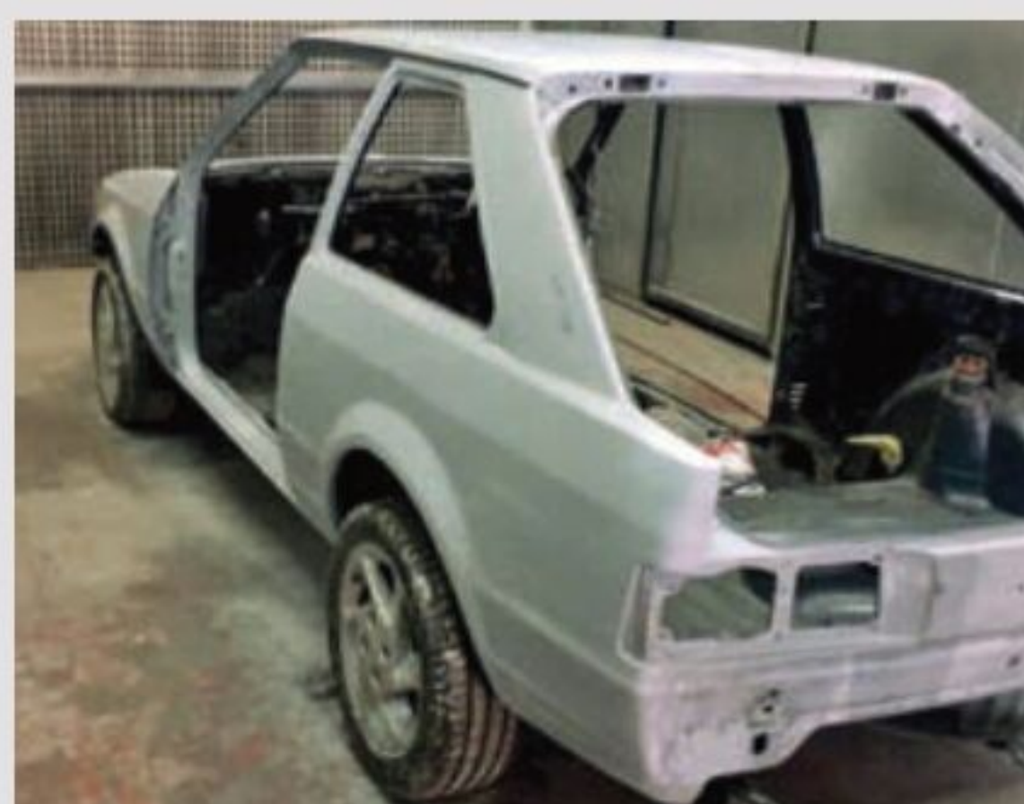
Once the rust had been cut out and fresh metal let in, the shell was taken to AB Paintworx for paint.
